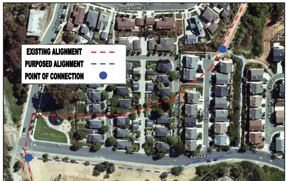
Santa Fe Avenue Force Main Realignment
