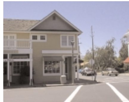
Build-to line - The building is built up to the edge of the sidewalk
